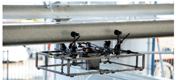
Beam UT measurement on top of tank
